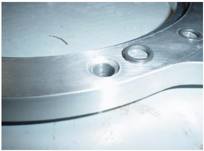
Figure 1 -- adapter bolt hole o-rings
