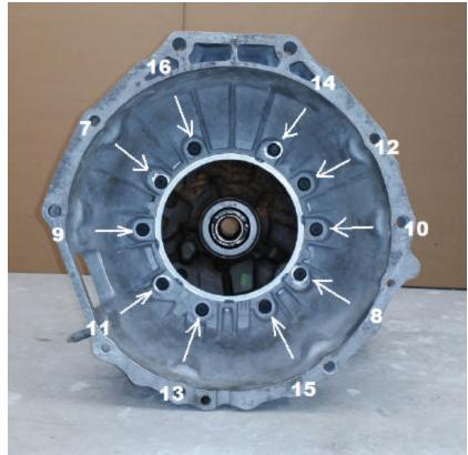
Figure 8 – bellhousing bolt torque sequence
