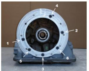
Figure 3 – Adapter installed, torque sequence
