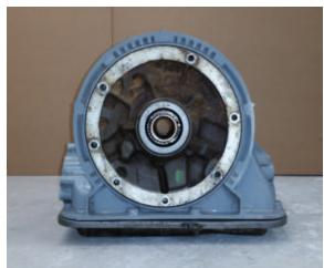
Figure 2 – Machined housing and pump face
